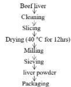
Fig 1: Flow Chart for the Production of Liver Powder
